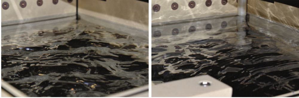
Fig. 1 Flows under consideration, exhibiting wave-like motion on the surface. A liquid metal is driven with the Lorentz force (see Sect. 3). Left highly fluctuating motion when the forcing is strong ( I = 400 A). Right with a gentle forcing ( I = 80 A), a linear wave is excited at 5 Hz from a corner of the container
